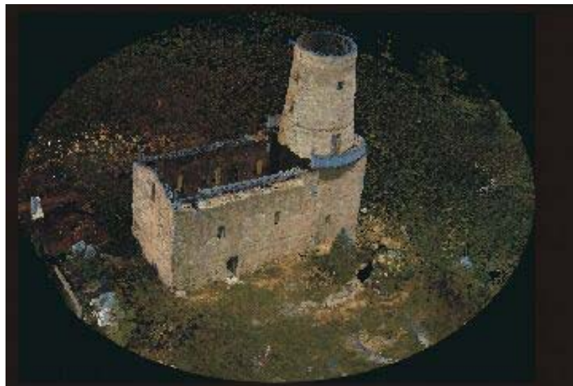
Figure 6: Left: RIEGL LMS-Z360 at work on a 4m high tripod to document the historical building. Right: 3D visualization of the acquired point cloud.
