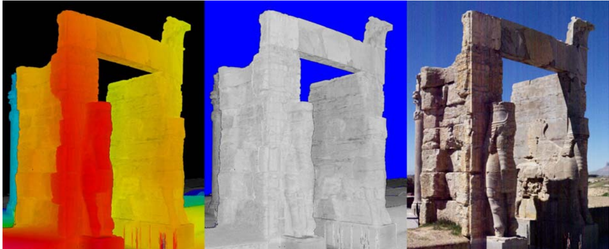
Figure 2: Example of the on-line visualization by 3D-RiSCAN from the survey at Persepolis, Iran.
