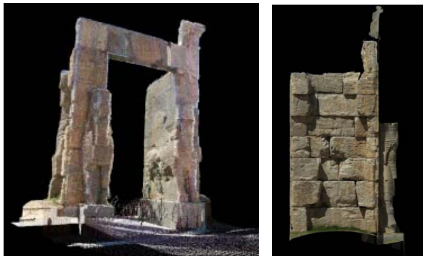
Figure 4: ‘Gate of All Nations’, left: point cloud of 9 true color scans, created semi-automatically whilst scanning right: orthophoto of merged scans and photographs
