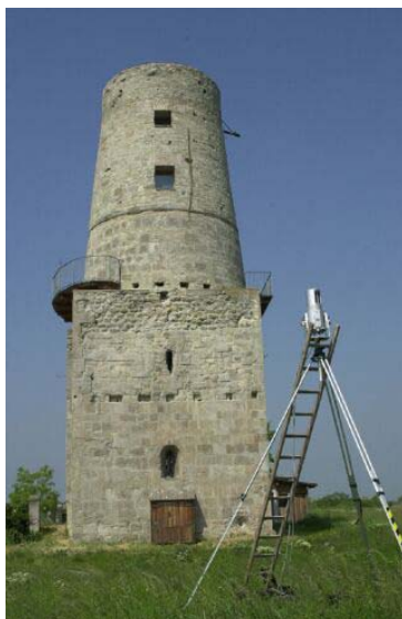
Figure 6: Left: RIEGL LMS-Z360 at work on a 4m high tripod to document the historical building. Right: 3D visualization of the acquired point cloud.
